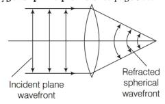
When a plane wavefront (parallel rays) is incident on a thin convex lens, the emergent rays are focused on the focal point of the lens. Thus, the shape of emerging wavefront is spherical. (2)
