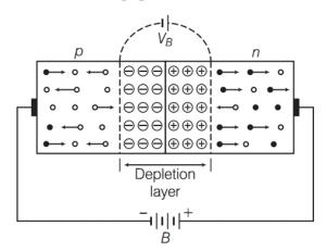
During the formation of *p-n* junction, diffusion of charge takes place. As, soon as *p*-type semiconductor is joined with *n*-type semiconductor, diffusion of free charges across the junction starts. (1)
