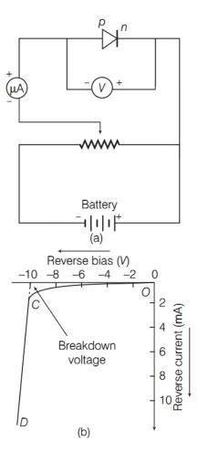
In reverse biased, the applied voltage supports the flow of minority charge carriers across the junction. So, a very small current flows across the junction due to minority charge carriers.
