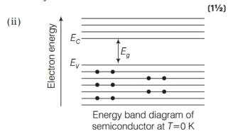
At absolute zero temperature (0 K), conduction band of semiconductor is completely empty, i.e.,  $\sigma$ =0.
