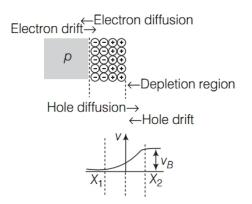
The accumulation of negative charges in the p-region and positive charge in the n-region sets up a potential difference across the junction. This acts as a barrier and is called barrier potential  $V_B$ .
