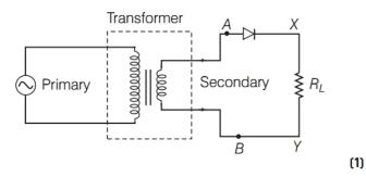
**Working** During positive half cycle of the input AC, the *p-n* junction is forward biased. Thus, the resistance in *p-n* junction becomes low and current flows. Hence, we get output in the load. During negative half cycle of the input AC, the *p-n* junction is reverse biased. Thus, the resistance of *p-n* junction is high and current does not flow. Hence, no output in the load. So, for complete cycle of AC, current flows through the load resistance in the same direction.
