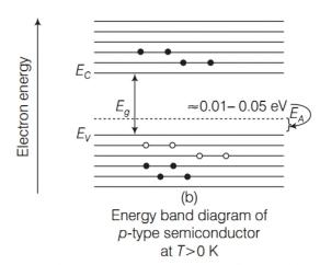
In *n*-type extrinsic semiconductors, the number of free electrons in conduction band is much more than the number of holes in valence band. The donor energy level lies just below the conduction band. In *p*-type extrinsic semiconductor, the number of holes in valence band is much more than the number of free electrons in conduction band. The acceptor energy level lies just above the valence band.
