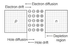
This sets up potential difference across the junction and an internal electric field  $E_i$  directed from n-side to p-side. The equilibrium is established when the field  $E_i$  becomes strong enough to stop further diffusion of the majority charge carriers (however, it helps the minority charge carriers to drift across the junction).
