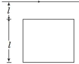
this loop is placed in a horizontal plane near a long straight conductor carrying a steady current  $I_1$  at a distance  $l$  as shown.
