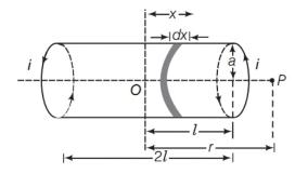
Let *i* be the current passing through a solenoid, *a* be the radius of solenoid, 2*l* be the length of solenoid and *n* be the number of turns per unit length of solenoid.
