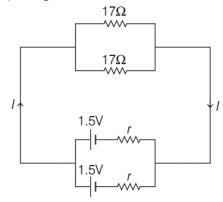
Resistance of external circuit = Total resistance of two resistances of 17  $\Omega$  connected in parallel
