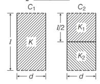
**23.** You are given an air filled parallel plate capacitor  $C_1$ . The space between its plates is now filled with slabs of dielectric constants  $K_1$  and  $K_2$  as shown in figure. Find the capacitance of the capacitor  $C_2$  if area of the plates is A and distance between the plates is d. Foreign 2011
