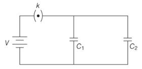
The key is now thrown open and a dielectric slab of dielectric constant K is inserted in the two capacitors to completely fill the gap between the plates. Find the ratio of
