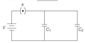
**13.** Find the charge on the capacitor as shown in the circuit. Foreign 2014
