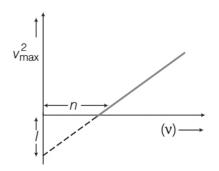
Light of frequency v incident is on a photosensitive surface. A graph of the square of the maximum speed of the electrons  $(v_{\text{max}}^2)$  versus v is obtained as shown in the figure. Using Einstein's photoelectric equation, obtain expressions for (i) Planck's constant and (ii) work function of the given photosensitive material in terms of parameters l, n and mass of the electron m. All India 2018C
