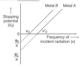
**6.** The graph shows variation of stopping potential  $V_0$  versus frequency of incident radiation v for two photosensitive metals A and B. Which one of the two metals has higher threshold frequency and why?
