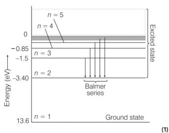
**50.** According to Bohr's postulates for hydrogen atom electron revolves in a circular orbit around the heavy positively charged nucleus. These are the stationary (orbits) states of the atom.
