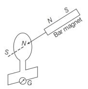
Figure shows a simple experiment to prove Lenz's law. When the North pole of the bar magnet is pushed towards the coil, the pointer in the galvanometer deflects indicating the presence of electric current in the coil. (1)
