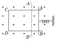
spring which is stretched to A' B' and then released at time t=0. Explain qualitatively how induced electro motive force in the coil would vary with time. (Neglect damping of oscillations of spring)
