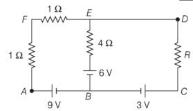
**28.** Calculate the value of the resistance *R* in the circuit shown in the figure, so that the current in the circuit is 0.2 A. What would be the potential difference between points *A* and *B*? All India 2012
