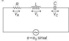
*L-C-R* circuit is said to in the resonance condition when current through it has maximum value. The frequency of AC at which current attains its peak value is called resonance frequency. L-C-R series
