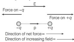
(b) E is increasing anti-parallel to p. So, the torque still remains zero, but the net force on the dipole will be in the direction of increasing electric field which is opposite to the dipole moment. Hence, it will have linear motion opposite to the dipole moment.
