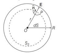
The electric flux through the Gaussian surface, as calculated in Eq. (i), i.e.  $E \times 4\pi r^2$ . As, charge inside a spherical shell is zero. So, the Gaussian surface encloses no charge. The Gauss' theorem gives
