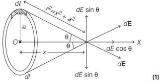
Let the total charge q is uniformly distributed, so the charge dq on element dl is  $dq = \frac{q}{2\pi a} \times dl$ .
