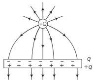
Electric lines of forces should fall normally on the surface of conductor, i.e. at 90° on the conducting plate. (2)
