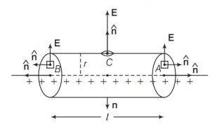
From symmetry, the electric field is everywhere in the radial direction and its magnitude only depends on the radial distance (r).
