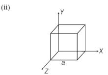
Since, the electric field has only x component. For faces normal to X-direction the angle between E and  $\Delta S$  is  $0^{\circ}$ . Therefore, the flux is separately zero for each of the cube except the surface perpendicular to X-axis.
