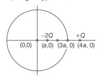
Charge enclosed by the sphere = -2QTherefore,  $\phi = 2Q/\epsilon_0$  (inwards) (1)
