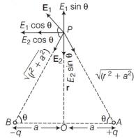
Electric field at point P due to charge -q,
