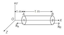
As the electric field is only along the X-axis, so flux will pass only through the cross-section of the cylinder.
