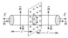
Flux through the flat surfaces = EA + EA = 2EAThe total electric flux over the entire surface of cylinder
