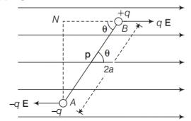
According to the figure, if we consider an electric dipole consisting of charges -q and +q of length 2a placed in a uniform electric field  $\mathbf{E}$  making an angle  $\theta$  with electric field, then force exerted on charge -q at A = -q  $\mathbf{E}$
