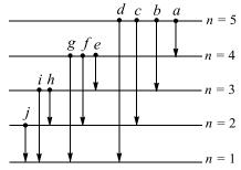
Transitions *a*, *e*, *h* and *j* can be performed by a single atom also. This is also true about transitions *b* and *i*, other transitions require one atom each
