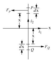
$F_P = B_1 i_2 dx = \frac{\mu_0 i_1 i_2}{2\pi x} dx$ , along *x*-axis Magnetic field at point *Q* due to  $i_1$  $B_2 = \frac{\mu_0 i_1}{2\pi x}$ , downward perpendicular to plane of paper.
