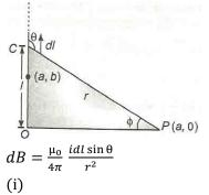
Here,  $\theta = 90^\circ + \phi$ ;  $r = a \sec \phi$ And  $l = a \tan \phi$ ;  $dl = a \sec^2 \phi d \phi$   $\therefore dB = \frac{\mu_0}{4\pi} \frac{i(\sec^2 \phi d \phi) \sin(90^\circ + \phi)}{a^2 \sec^2 \phi}$   $= \frac{\mu_0}{4\pi} \frac{1}{a} \cos \phi d \phi$ Total magnetic field induction at *P* is
