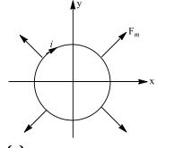
In adjoining loops of spring, the current being in the same direction, there will be attraction. Due to which the spring gets compressed.
