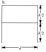
In the given case the two capacitors are in parallel.  $C' = C_1 + C_2$
