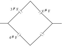
The effective capacitance in upper arm in series, is given by
