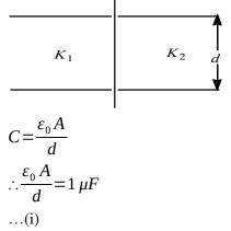
When it is filled with dielectric of dielectric constant  $K_1 \wedge K_2$  as shown, then there are two capacitors connected is parallel. So,
