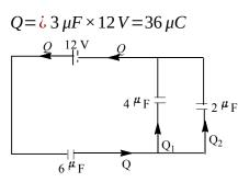
Since, the capacitors  $4 \mu F$  and  $2 \mu F$  are connected in parallel, therefore potential difference across them is same.
