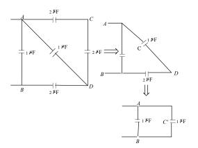
The capacitors  $2\mu F$  and  $2\mu F$  of arm ACD are in series. So, their equivalent capacitance is  $1\mu F$  which is in parallel with capacitor of  $1\mu F$  of arm AD. So, equivalent capacitance now is  $2\mu F$ . This capacitance is now in series with  $2\mu F$ capacitance of arm BD which equivalents to  $1\mu F$  is in parallel with  $1\mu F$  capacitance of arm AB. So, final effective capacitance= $2\mu F$ .
