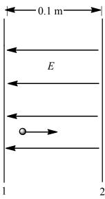
Use work-energy theorem to find speed of electron when it strikes the plate 2.
