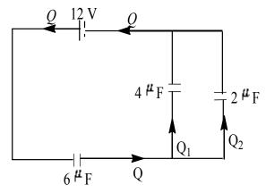
As the capacitors 4  $\mu F$  and 2  $\mu F$  are connected in parallel and are in series with  $6\mu F$  capacitor, their equivalent capacitance is
