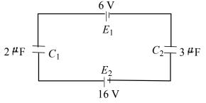
Net emf in the circuit here  $E = E_2 - E_1 = 16 - 6 = 10$  volt While the equivalent capacity
