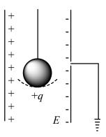
when it is suspended between vertical plates of a charged parallel plate capacitor, then acceleration due to electric field,
