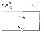
$\therefore$ Capacitors are in parallel, in parallel  $V_0$  is same for all capacitors.
