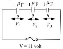
Then,  $V = \frac{q}{C_1}$ ,  $V_2 = \frac{q}{C_2}$ ,  $V_3 = \frac{q}{C_3}$ The total potential difference V = 11 volt  $\therefore V = V_1 + V_2 + V_3$   $\Rightarrow V = \frac{q}{C_1} + \frac{q}{C_2} + \frac{q}{C_3} = 11$ Given,  $C_1 = 1\mu F$ ,  $C_2 = 2\mu F$ ,  $C_3 = 3\mu F$   $\therefore 11 = q\left(\frac{1}{1} + \frac{1}{2} + \frac{1}{3}\right)$   $\Rightarrow 11 = \frac{11q}{6}$   $\Rightarrow q = 6\mu c$  $\therefore V_1 = \frac{q}{C_1} = \frac{6}{1} = 6V$
