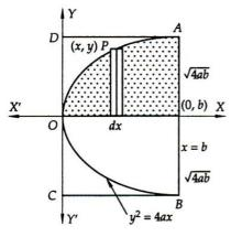
And,  $A_2$  = Area of the rectangle *ABCD*   $\Rightarrow A_2 = AB \times AD = 2\sqrt{4ab} \times b = 4 a^{1/2}b^{3/2}$   $\therefore A_1 : A_2 = 8/3 a^{1/2}b^{3/2} : 4 a^{1/2}b^{3/2} = 2/3 : 1$ = 2 : 3
